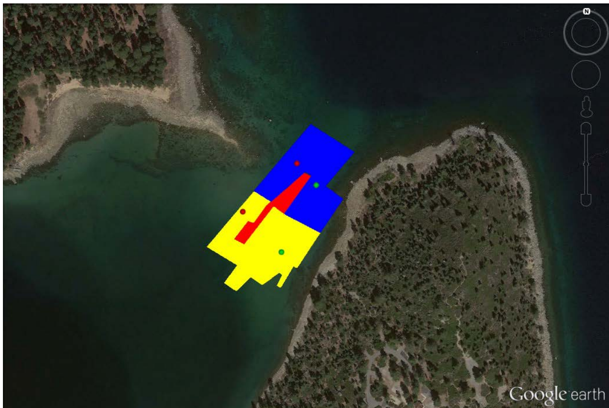
Figure 7. Aerial image of the Emerald Bay sill area with color polygons showing the approximate location of the three benthic barrier treatment categories. The blue polygon defines the approximate area of undisturbed benthic barriers over substrate with reduced permeability. The yellow polygon defines the approximate area of undisturbed benthic barriers over substrate with enhanced permeability. The red polygon defines the approximate area of disturbed benthic barriers. The red and green dots represent the approximate locations of the channel navigation buoys. See Figure 10 for the locations of intentionally moved benthic barriers.
