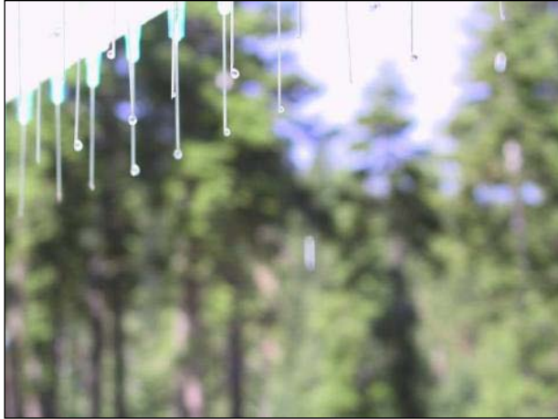
Figure 1. Rain drops are generated from more than 800 hypodermic needles on the rainfall simulator.
