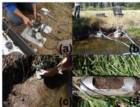
Fig. 5. Field instrumentation for measuring bank properties. (a) Borehole Shear Tester (BST) for measurement of soil cohesion; (b) Jet Test for erodibility and critical shear stress; (c) Cohesive Strength Meter (CSM) for critical shear stress; (d) soil sample for density, moisture, and composition.
